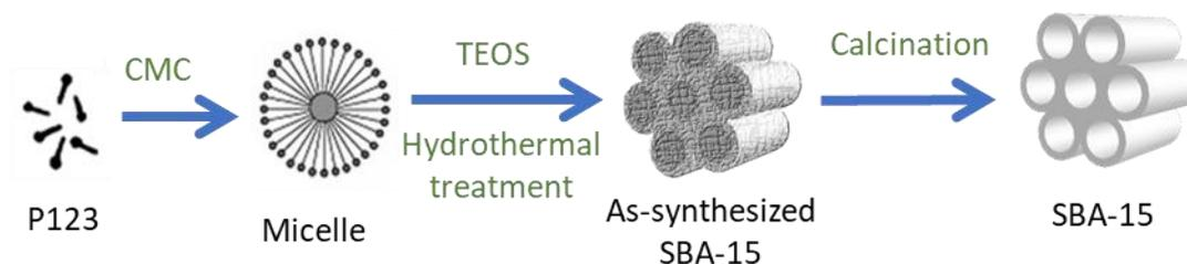
**Scheme S1.** A generalized representation of the formation of ordered mesoporous Silica (SBA-15) by liquid crystal templating method.
