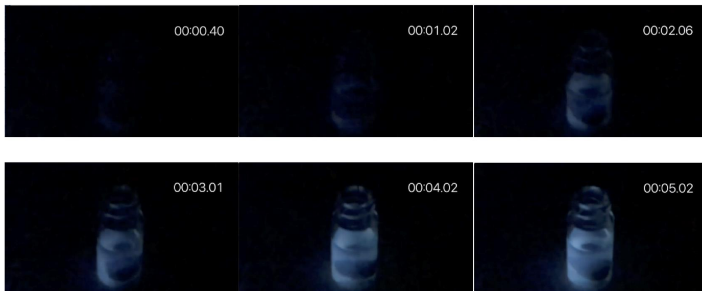
Figure 3. Appearance of fluorescence when ascorbic acid solution was added to a solution of compound 5 in MeOH. The top row from left to right: pictures after 0 sec., 1 sec., and 2 sec. The bottom row from left to right: pictures after 3 sec., 4 sec., and 5 sec.
