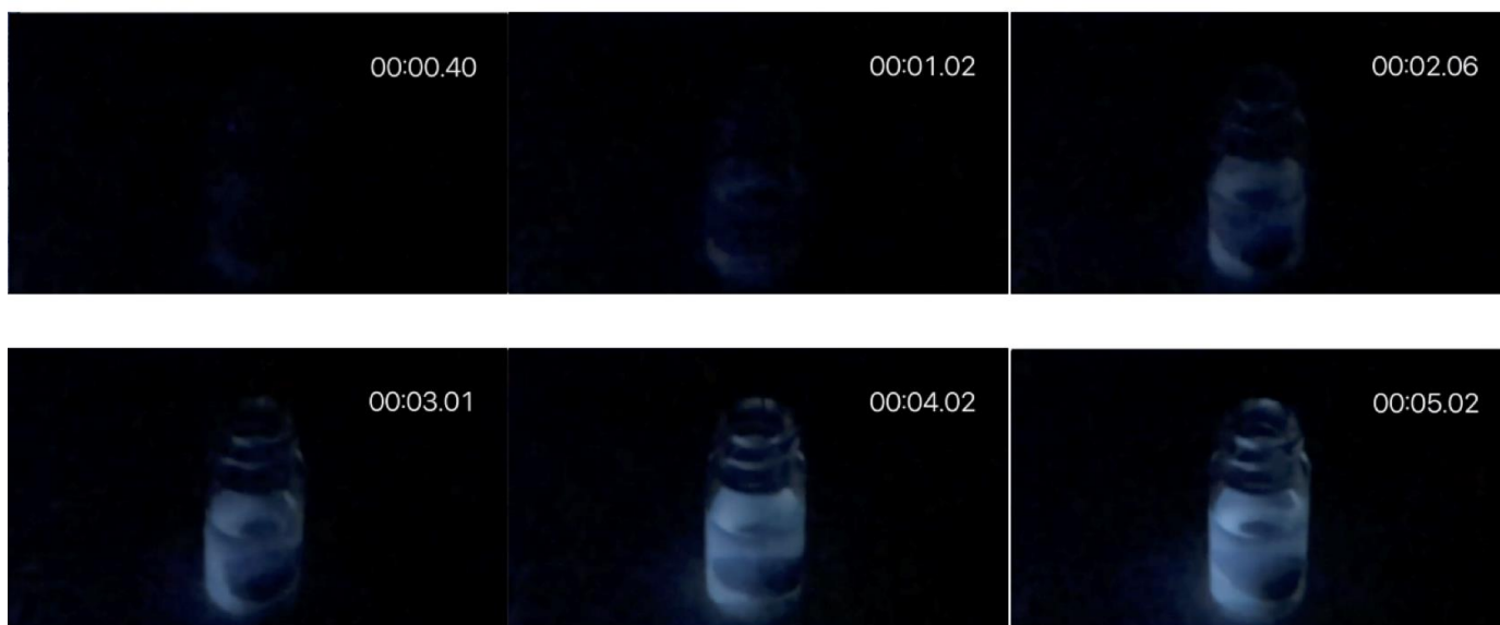
Figure 3. Appearance of fluorescence when ascorbic acid solution was added to a solution of compound 5 in MeOH.
