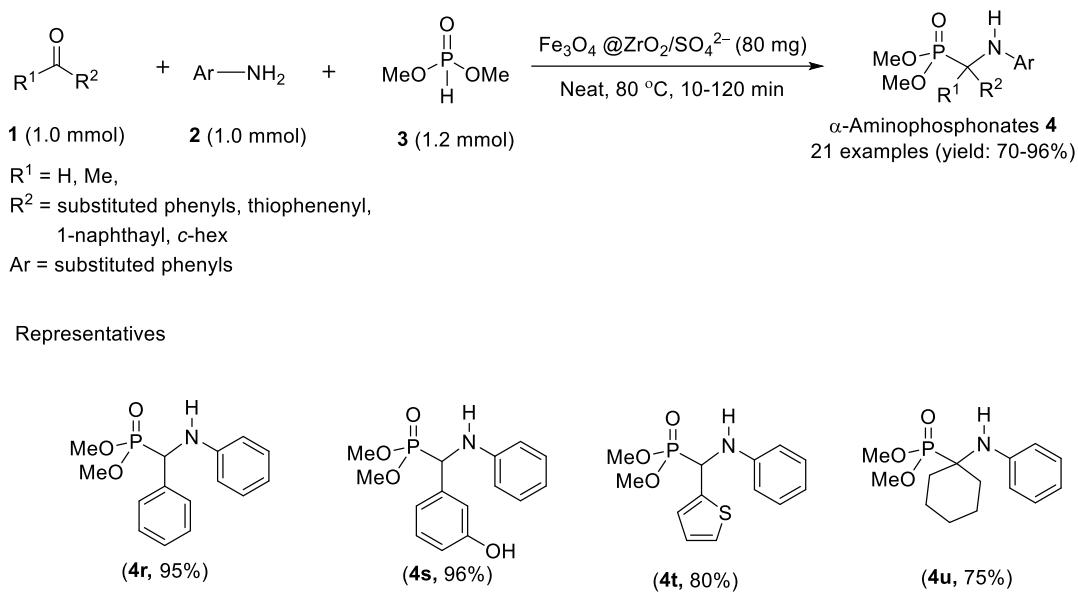
**Scheme 6.** Nanomagnetic sulfated zirconia-catalyzed synthesis of  $\alpha$ -aminophosphonates under heating
