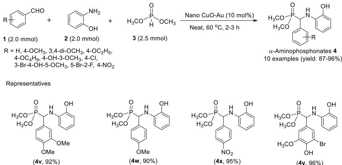
**Scheme 8.** Nano CuO-Au-catalyzed synthesis of  $\alpha$ -aminophosphonates under heating
