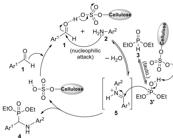
**Scheme 2b.** The suggested mechanism of cellulose-SO<sub>3</sub>H catalyzed synthesis of  $\alpha$ -aminophosphonates **4**
