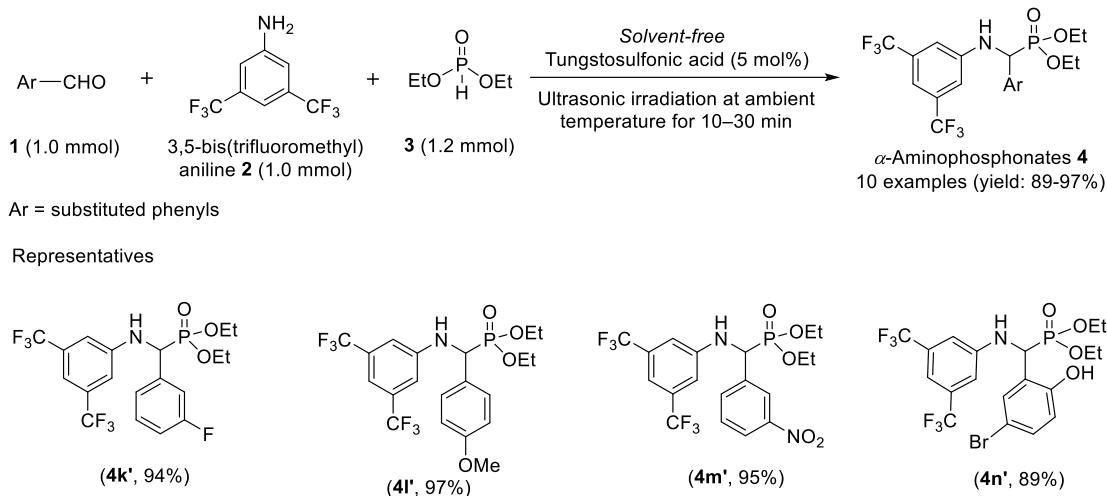
**Scheme 14.** Tungstosulfonic acid-catalyzed synthesis of  $\alpha$ -aminophosphonates under ultrasonication
