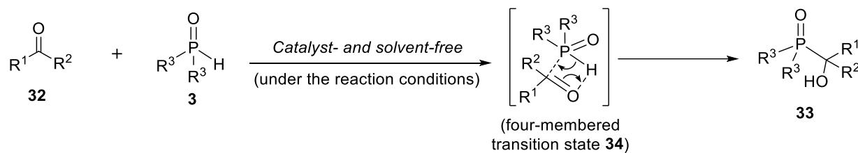
**Scheme 28.** Proposed synthetic pathway for tertiary  $\alpha$ -hydroxyphosphine oxides
