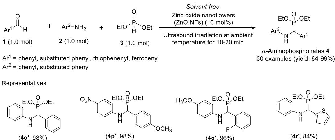
**Scheme 15.** ZnO NFs-catalyzed synthesis of  $\alpha$ -aminophosphonates under ultrasonication
