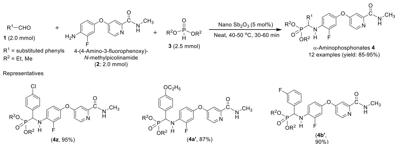
**Scheme 9.** Nano  $Sb_2O_3$ -catalyzed synthesis of  $\alpha$ -aminophosphonates under heating
