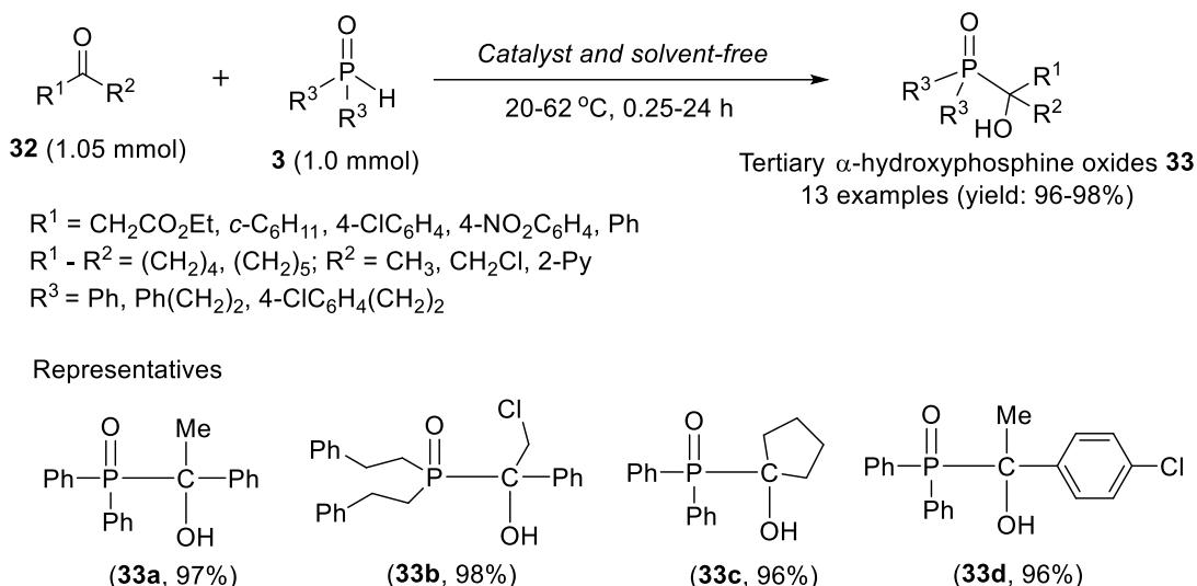
**Scheme 27.** Catalyst- and solvent-free synthesis of tertiary  $\alpha$ -hydroxyphosphine oxides
