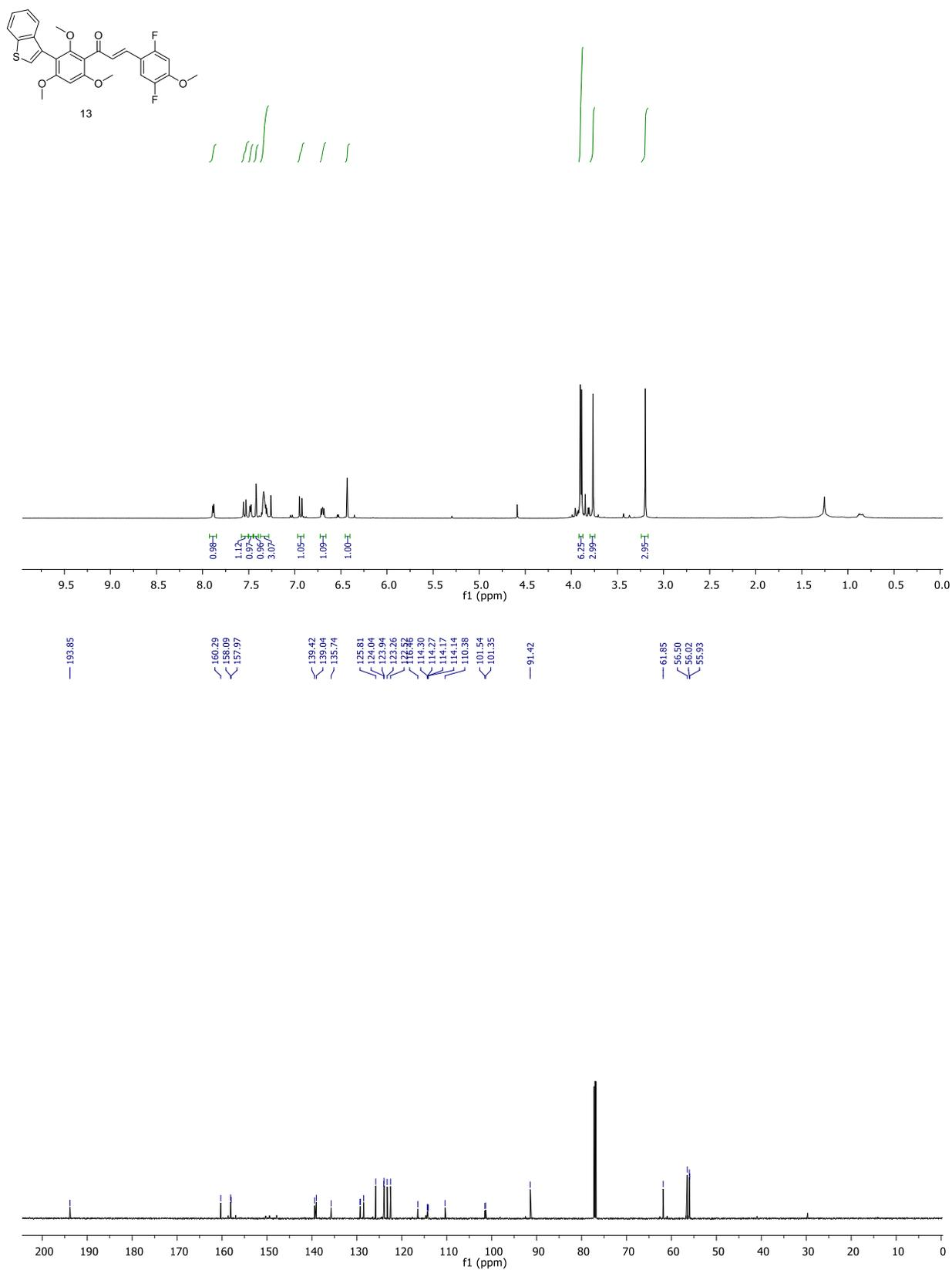
S12.  $^1\text{H}$  and  $^{13}\text{C}$  spectra of (*E*)-1-(3-(benzo[*b*]thiophen-3-yl)-2,4,6-trimethoxyphenyl)-3-(5-fluoro-2,4-dimethoxyphenyl)prop-2-en-1-one (**14**)
