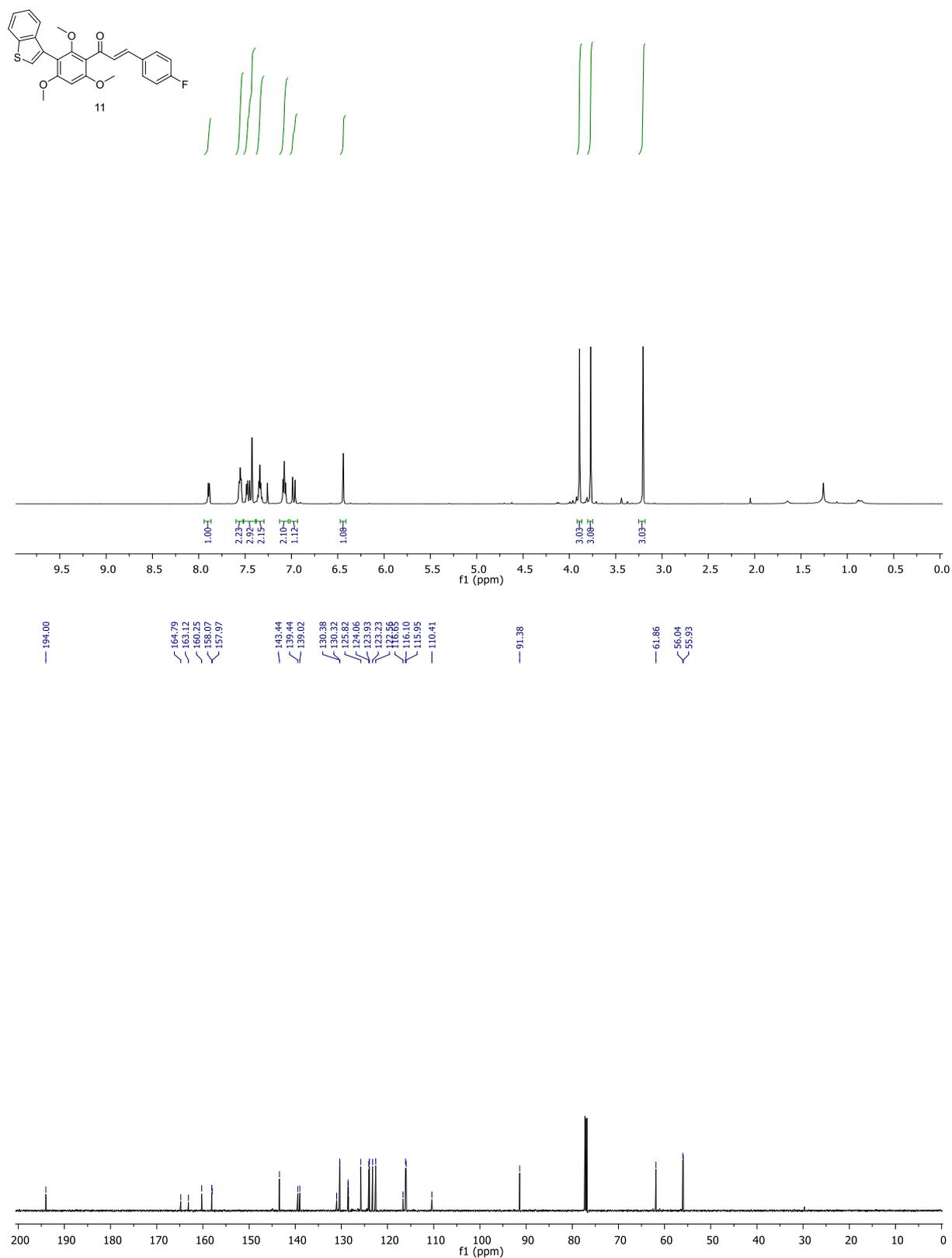
S10.  $^1\text{H}$  and  $^{13}\text{C}$  spectra of (*E*)-1-(3-(benzo[*b*]thiophen-3-yl)-2,4,6-trimethoxyphenyl)-3-(4-methoxyphenyl)prop-2-en-1-one (**12**)
