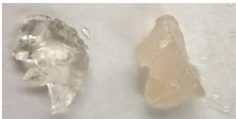
Figure 5. Image of CMC gels with a low (20:1) CMC: \text{CaCl}_2 ratio (left) and a high (1:1) ratio (right). It is clear that at high electrolyte concentrations CMC gels are more heterogenous and chains start to precipitate, with increased opacity of the corresponding materials.
