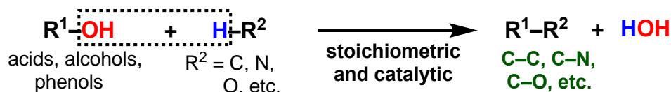
Scheme 1. Dehydrative C–heteroatom bond construction
