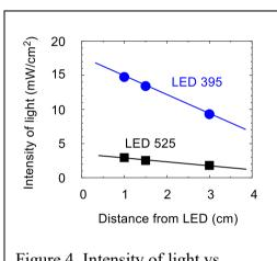
Figure 4. Intensity of light vs distance from LED
