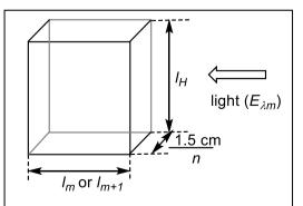
Figure 3. Rectangular parallelepiped of the solution at *m* th segment
