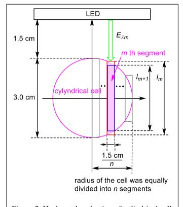
Figure 2. Horizontal projection of cylindrical cell
