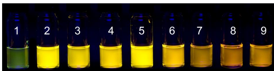
Figure 3. Emission colors of derivative 5 in various solvents; \lambda_{\text{ex}} = 366 \text{ nm} . 1: \text{H}_2\text{O} , 2: 2-PrOH, 3: AcOH, 4: EtOH, 5: 1-BuOH, 6: THF, 7: MeOH, 8: MeCN, 9: DMSO.
