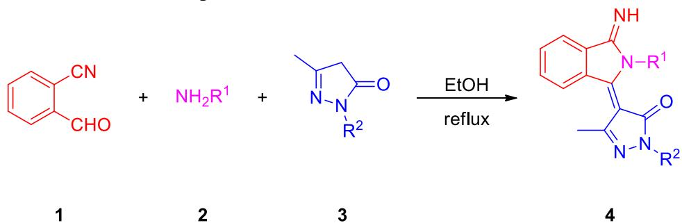
**Scheme 1.** Synthesis of 4-(2-substituted-3-iminoisoindolin-1-ylidene)-1 substituted-3-methyl-1*H*-pyrazol-5(4*H*)-ones **4**
