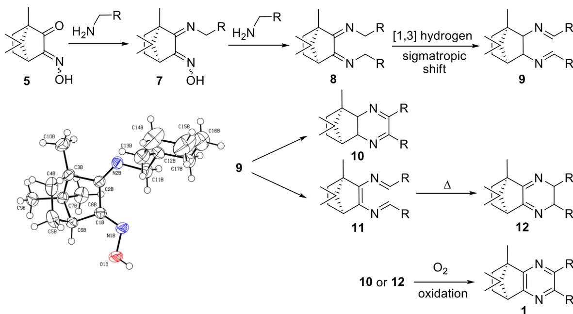
**Scheme 2.** Proposed reaction path of the condensation between monooximes and amines and the ORTEP plot of **7** (R = cyclohexyl).
