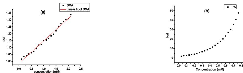
**Figure 3.** Stern-Volmer plots for the fluorescence quenching of **2b** with a) DMA and b) PA.
