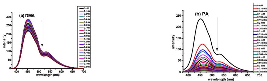
**Figure 2.** Steady state fluorescence spectra of **2b** in the presence of increasing concentration of quencher a) DMA and b) PA.
