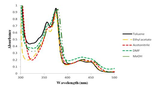
**Figure 4.** Visible absorption spectra of compound **3c** in different solvents  $(1 \times 10^{-6} \text{ mol } \text{L}^{-1})$ .
