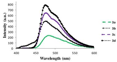
**Figure 3.** Emission spectra of compounds **3a-d** in DCM solution  $(3 \times 10^{-7} \text{ mol L}^{-1})$ .
