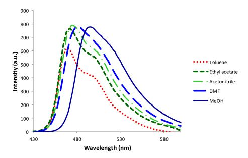
**Figure 5.** Emission spectra of compound **3c** in some solvents  $(5 \times 10^{-7} \text{ mol } \text{L}^{-1})$ .
