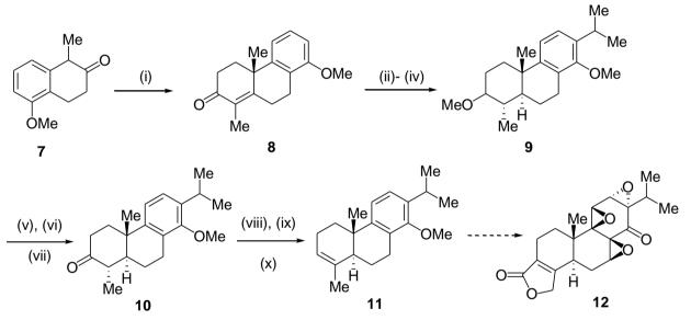
Reagents: (i) 1-chloro-3-pentanone; (ii) Na, *n*-propanal; (iii) MeI, NaH, THF; (iv) isopropanal, PPA; (v) MeSiCl, NaI, MeCN; (vi) CrO<sub>3</sub>, H<sub>2</sub>SO<sub>4</sub>; (vii) Me<sub>2</sub>SO<sub>4</sub>, K<sub>2</sub>CO<sub>3</sub>, Me<sub>2</sub>CO; (viii) NaBH<sub>4</sub>, MeOH; (ix) TsCl/ Py; (x) Li<sub>2</sub>CO<sub>3</sub>, DMF
