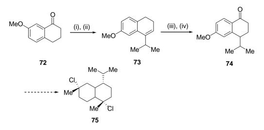
Reagents: (i) i-PrMgCl, CeCl<sub>3</sub>, THF, 0  $^{\circ}$ C; (ii) PTSA, C<sub>6</sub>H<sub>6</sub>; (iii) H<sub>2</sub>, Pd-C 10%, 1 atm; (iv) 10% CrO<sub>3</sub>-AcOH
