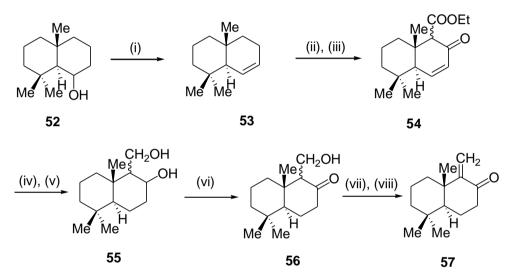
Reagents: (i) PTSA, silica gel; (ii) CrO<sub>3</sub>, Py, 3,5dimethylpyrazole; (iii) DME, CO(COOEt)<sub>2</sub>, NaH; (iv) PtO<sub>2</sub>, MeOH; (v) LiAlH<sub>4</sub>, THF; (vi) NaClO<sub>4</sub>, MeCOOH, (vii) TsCl, Py; (viii) 1,5-diazabicyclo[5.4.0]-undec-5-ene
