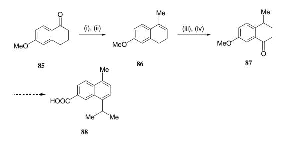
Reagents: (i) MeMgBr; (ii) HCl, 6N; (iii) H<sub>2</sub>, Pd/ C(10%); (iv) 10% CrO<sub>3</sub> - CH<sub>3</sub>CO<sub>2</sub>H
