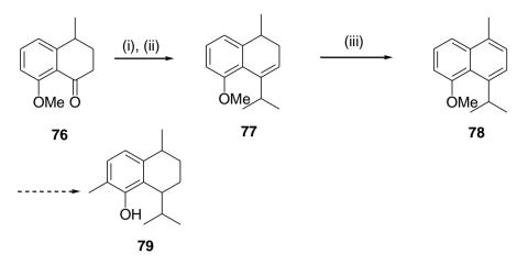
Reagents: (i) *i*-PrMgCl, THF, 0 <sup>0</sup>C; (ii) HCl, 6N; (iii) DDQ, CH<sub>2</sub>Cl<sub>2</sub>
