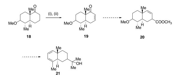
Reagents: (i) C<sub>5</sub>H<sub>6</sub>NBr<sub>3</sub>, EtOH, CHCl<sub>3</sub>; (ii) LiBr, Li<sub>2</sub>CO<sub>3</sub>, DMF
