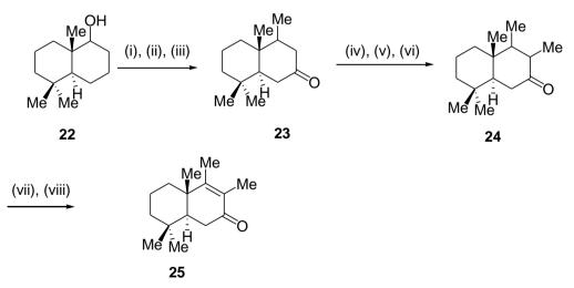
Reagents: (i) PTSA on silica gel, CHCl<sub>3</sub>; (ii) CrO<sub>3</sub>, 3,5-DMP; (iii) MeLiCu<sub>2</sub>; (iv) CO(COOEt)<sub>2</sub>, NaH, DME; (v) DMF, NaH, MeI, MeCOOH; (vi) DMSO, LiCl, H<sub>2</sub>O, 170 - 180 °C; (vii) Br<sub>2</sub>, CHCl<sub>3</sub>, MeCOOH; (viii) LiBr, Li<sub>2</sub>CO<sub>3</sub>, DMF
