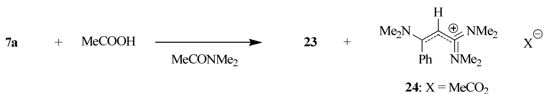
Scheme 8. Cleavage of 1,1,1-tris(dimethylamino)-3-phenyl-2-propyne ( 7a ) by acetic acid.
