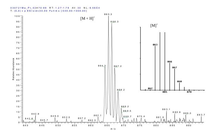
**Figure 6.** Positive-ion electrospray mass spectrum of complex **14ggg** in CH<sub>3</sub>CN/H<sub>2</sub>O (70/30) + 0.05% TFA. The inset shows the calculated isotope pattern for the  $[M]^+$  ion (*m*/*z* 864).
