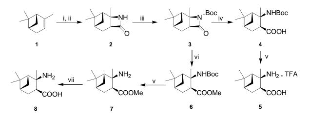
**Scheme 1.** (i) CSI, diethyl ether, 1 h, rt., (ii) Na<sub>2</sub>SO<sub>3</sub>/H<sub>2</sub>O, then KOH, 76%;<sup>14</sup> (iii) (Boc)<sub>2</sub>O, Et<sub>3</sub>N, DMAP/THF, rt., 12 h, 89%; (iv) LiOH/H<sub>2</sub>O, rt., 7 h, 78%; (v) TFA/CH<sub>2</sub>Cl<sub>2</sub>, rt., 4 h, 96%; (vi) cat. NaOMe/MeOH, rt., 0.5 h, 92%; (vii) dioxane/H<sub>2</sub>O, reflux, 48 h, 85%.
