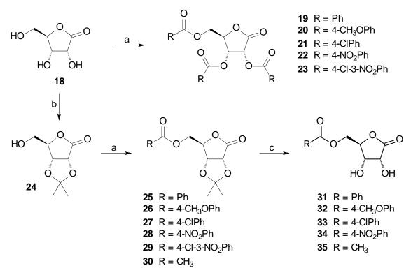
Conditions: a. RCOCI, py, rt (for **19-23**: 82-95%; for **25-29**: 80-99%) or Ac<sub>2</sub>O, py, rt (for **30**: 90%); b. Me<sub>2</sub>CO, HCI, rt (88%); c. TFA-H<sub>2</sub>O (1:1), 40°C or AcOH-H<sub>2</sub>O (1:9), 90°C (54-99%).
