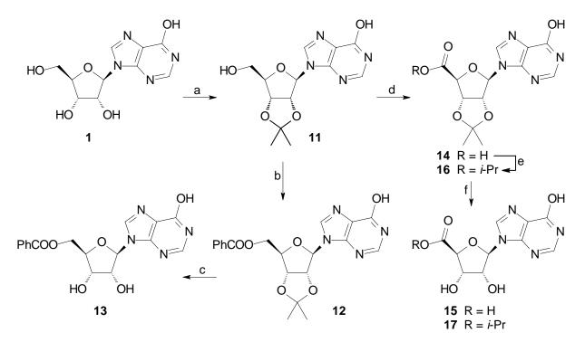
Conditions: a. *p*-TsOH, Me<sub>2</sub>CO, rt (66%); b. PhCOCI, py, 60°C (78%); c. AcOH-H<sub>2</sub>O (1:9), 90°C (68%); d. CrO<sub>3</sub>, AcOH, rt (58%); e. SOCI<sub>2</sub>, (CH<sub>3</sub>)<sub>2</sub>CHOH, rt (71%); f. 1M HCI, 80°C (70-75%).
