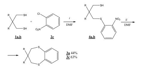
Reaction conditions: *i* NaHCO<sub>3</sub>, <u>**1a**</u> 50°C, 7h; NaHCO<sub>3</sub>, <u>**1b**</u> 60°C 7h. *ii* KOH, <u>**1a**</u> 50°C, 1h; <u>**1b**</u> 60°C, 1,5.
