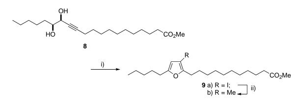
Scheme 3. Reagents: i)  $3NaHCO_3$ , alkyne-diol 8, dry EtOAc,  $20^{\circ}C$ , add  $3l_2$ ,  $20^{\circ}C$ , 1 h (93%); ii) Me<sub>4</sub>Sn, (Ph<sub>3</sub>P)<sub>4</sub>Pd (cat.), Cul (cat.), *N*-methylpyrrolidine, 65°C, 16 h (sealed tube) (57%).
