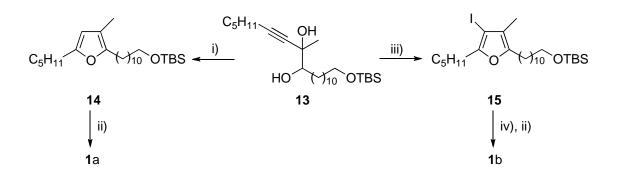
**Scheme 5.** *Reagents:* i) 10 mol% of 10 % AgNO<sub>3</sub>-SiO<sub>2</sub>, CH<sub>2</sub>CI<sub>2</sub>, 20 °C, 5 h (97%); ii) TBAF, THF, 20 °C, 1.5 h (90 %) then 5 PDC, Celite, DMF, 20 °C, 8 h (85%); iii) as i), Scheme 3, (87%); iv) BuLi, THF, -78 °C, 5 min then Mel (90%).
