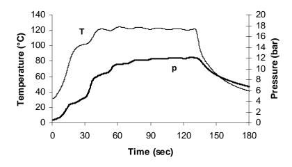
Figure 1. Temperature (T) and pressure (p) profiles for the reduction of DHPM  $7 \rightarrow 8$  under sealed vessel/microwave irradiation conditions.<sup>a</sup>
